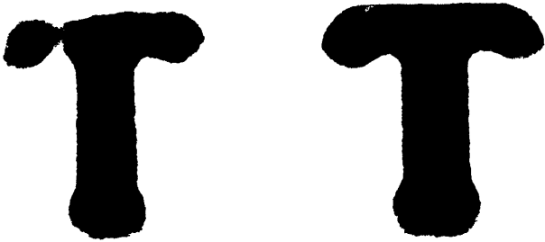
Figure 22. A pictorial description of the influence of defocusing or blurring on a typical and a perfect letter. The blurred images are more nearly alike.
