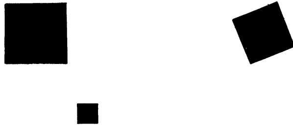
Figure 3. Typical characters which should be identified as similar by a form-perceiver which is not affected by size or orientation.
