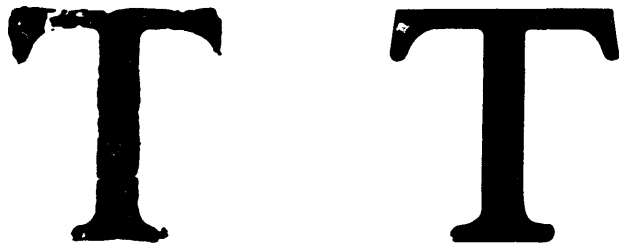
Figure 21. A typical enlarged character, originally set in 12 point type, and illustrating characteristic irregularity of outlines.
